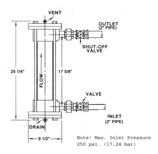
For maximum efficiency, the 8060601 Carbon Dioxide Filter unit should be installed as indicated in the above diagram. The unit should be installed in a vertical position only and the air flow must be in an upward direction only.
