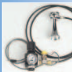
8039601 Air Horn Alarm System is used for explosive atmospheres. Operating pressure 20-30 PSI using a 100 PSI regulator.
